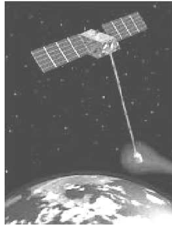
Figure 1 – Terminator Tether deorbit system
