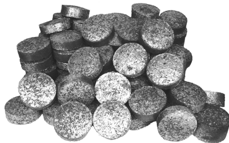
Fig. 3 – Appearance of multifunction modifiers of brand of one size Apparently from tab. 1, after modifying chemical composition of KP-T steel was stabilized. For establishment of the reasons of stabilization of chemical composition system thermodynamic researches on possible influence of components of special modifiers at their interaction with fusion are conducted.
