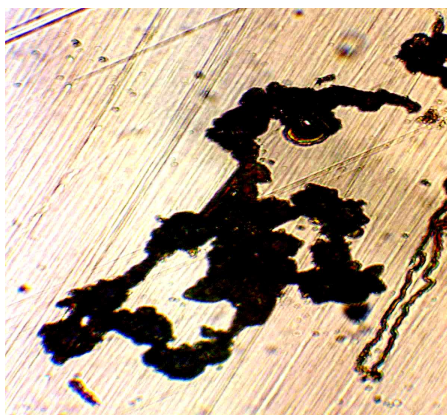
Fig. 1 – Disclosure of the microcrack formed on non-metallic inclusions with allocation products of atmospheric corrosion in KP-T steel. Allocations are from right to left visible products of atmospheric corrosion. White points in a crack - nonmetallic inclusions., x1000
